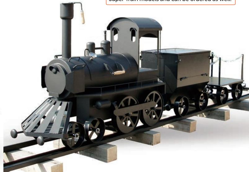
This Smoky Fun Super Train was built upon special order in 2013. The locomotive and the tender go together with rails and a trailer with a protective cover. The trailer is equipped with rails to facilitate transportation as well as with an electrical winch for easy loading and unloading.
